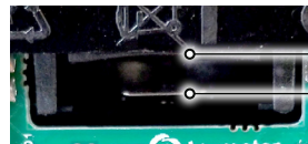
Install Battery Between These Two Points
