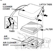
Remove and clean cartridge yearly or after every 25 hours, whichever occurs first. Service more often if necessary. Clean by tapping gently on flat surface. If very dirty, replace the cartridge using only original equipment parts available at any engine service center.
