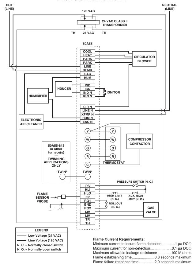
① Measured with a DC microammeter in the flame probe lead
