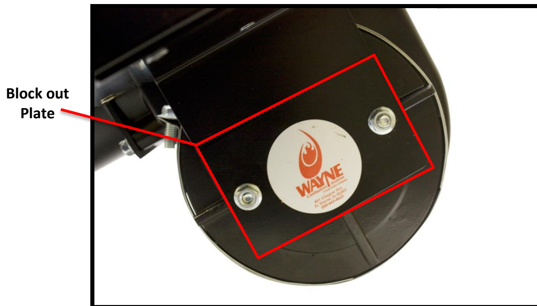
Block out plate location
