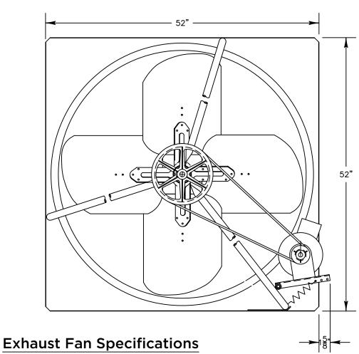
Blade Diameter: 48" Motor Enclosure: ODP
