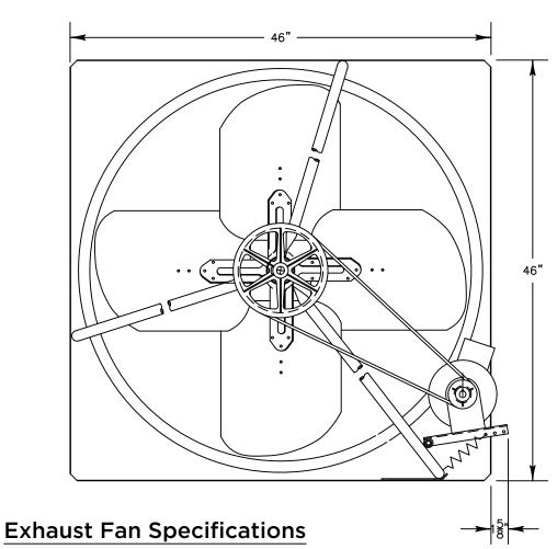
Blade Diameter: 42" Motor Enclosure: ODP
