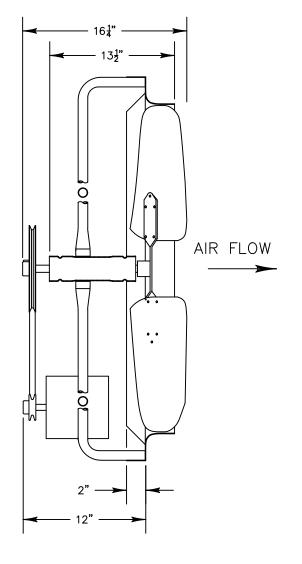
Motor Enclosure: TEFC Blade Diameter: 36"
