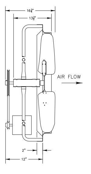
ODP **Motor Enclosure:** Blade Diameter: 36"
