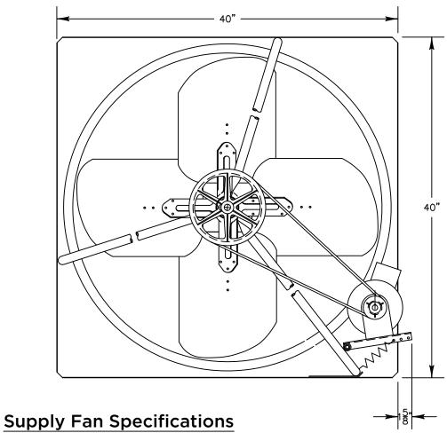
Blade Diameter: 36" Motor Enclosure: TEFC
