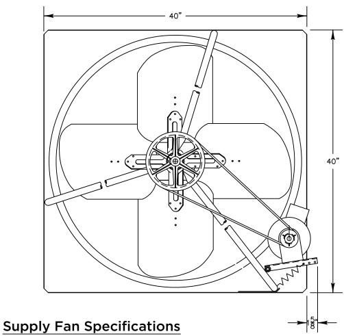
Blade Diameter: 36" Motor Enclosure: ODP
