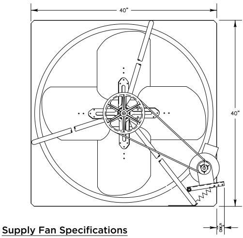
Blade Diameter: 36" Motor Enclosure: ODP
