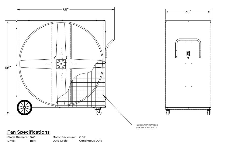
Horsepower: 2 Voltage: 115 Phase: 1 RPM: 615
