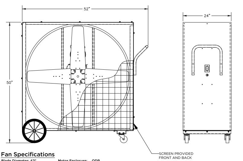
Blade Diameter: 42" Motor Enclosure: ODP
