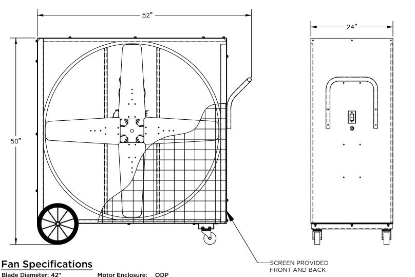
Blade Diameter: 42" Motor Enclosure: ODP
