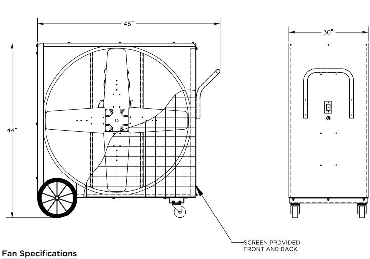
Blade Diameter: 36" Motor Enclosure: ODP
