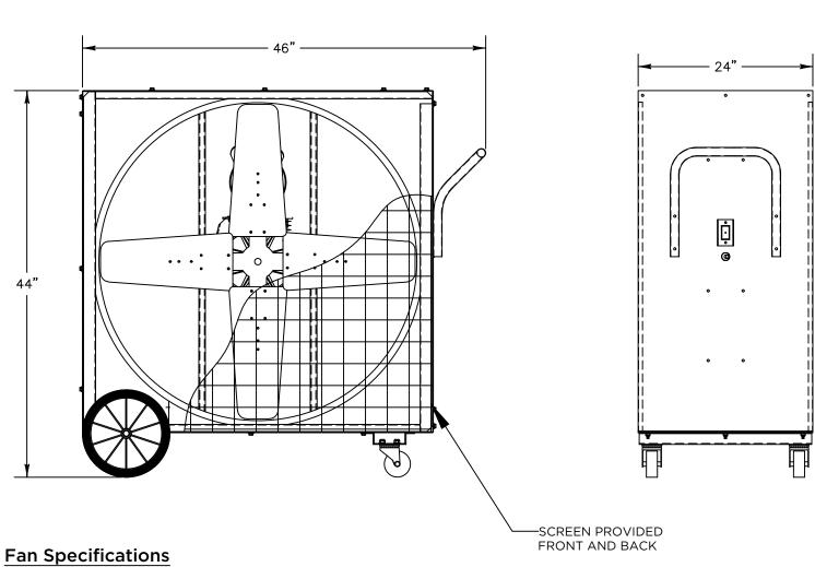
Blade Diameter: 36" Motor Enclosure: ODP
