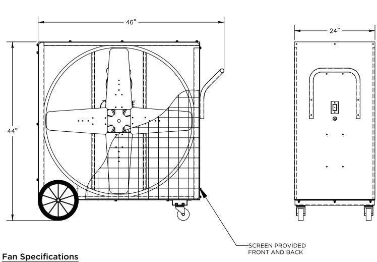
Blade Diameter: 36" Motor Enclosure: ODP
