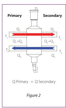
supply water temperature will be the same as a boiler or chiller primary circuit supply water temperature.
