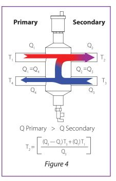
This can cause system performance problems, especially in chilled water systems, since the building secondary supply water temperature cannot be maintained at the chiller primary supply water temperature.
