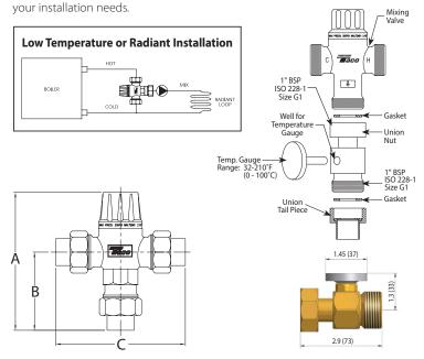
**5000 Series Heating Only Mixing Valve Dimensions** Dimensions for reference only
