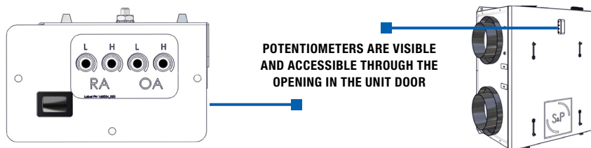
FIGURE 4.6.1 FAN SPEED CONTROL POTENTIOMETERS
