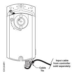
Figure 22. Input Cable Installed in Bottom Three Contacts.
