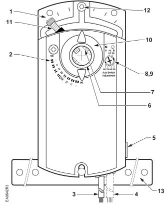
Figure 10. Parts of the Actuator.
