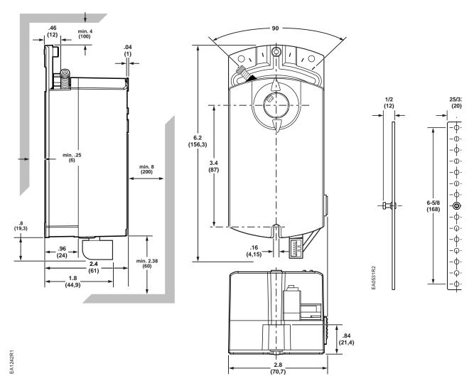
Figure 26. GDE131.1T, GDE131.1N, and Mounting Bracket Dimensions in Inches (Millimeters).
