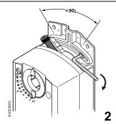
Figure 16. Moving the Mechanical Range Stop.
