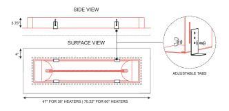
WARNING: Frame and heaters cannot be mounted on a sloped/pitched ceiling. Frame is only to be used on a flat, non-sloped ceiling. Flush mount applications must always be installed with heaters horizontal to the floor
