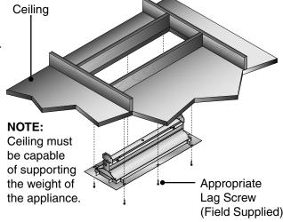
Figure 3 • Recessed Mount - Assembled
