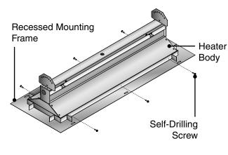
Figure 2 • Insert into Ceiling
