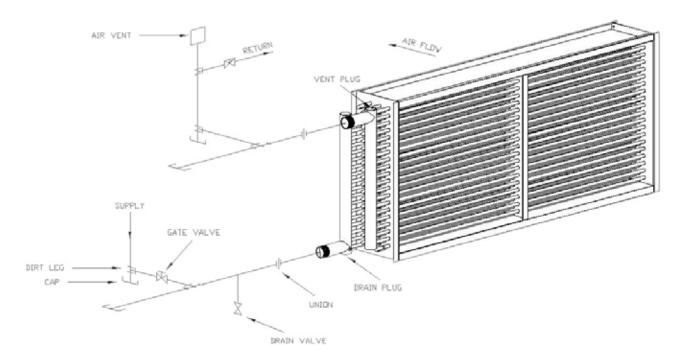
COLL PIPING VERTICAL AIR FLOW (RECOMMENDED FOR HOT WATER/GLYOL COILS ONLY)
