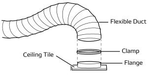
Remove the original ceiling tile and install the ceiling tile with duct. Use the tabs with holes to secure the tile in place in case ceiling T-bar is too narrow or weak.
