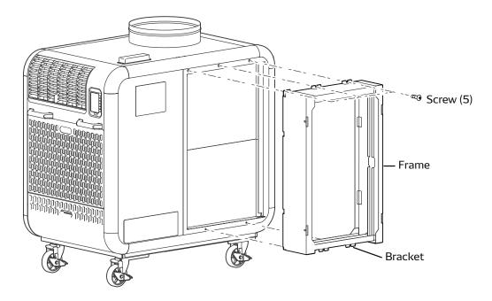
4. Insert the four (4) brackets of the plenum into the slots of the frame and secure the plenum to the frame with the four (4) bolts, which were removed in step 1 on page 2.
