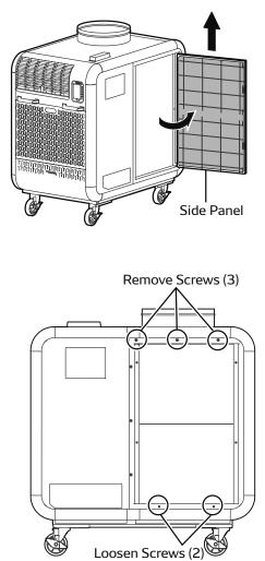
Loosen the bottom two (2) screws and remove the three (3) screws from the side of the unit.
