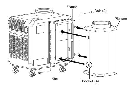
5. Remove the two (2) knob bolts and remove the plate from the plenum by lifting upward.
