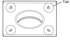
3. Place the other duct end over the flange on top of the unit or plenum. Secure the duct with the clamp.
