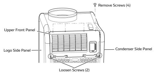
5. Remove the four (4) screws from the upper front panel.
