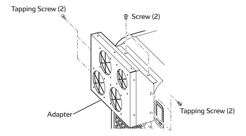
8. Secure the adapter to the frame with the four (4) screws.
