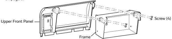
Reinstall the upper front panel, which was removed in step 4 on page 2.
