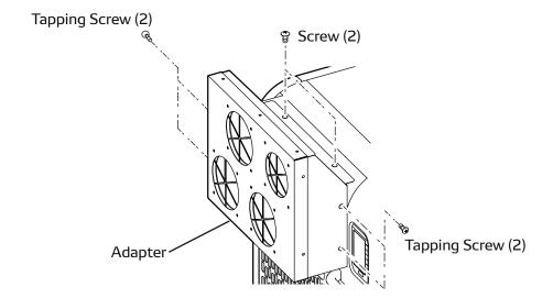
8. Attach the cold air flange to the adapter with the four (4) screws.
