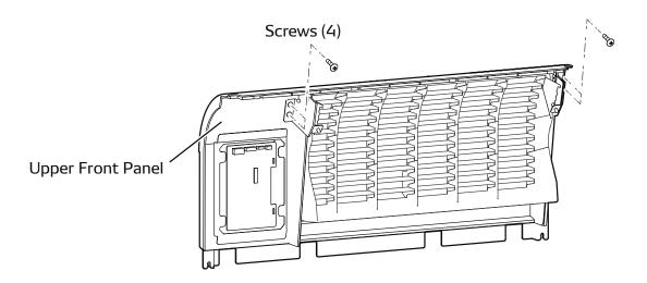
6. Remove the two (2) screws from the upper front panel. Remove the louver with the two (2) support plates.
