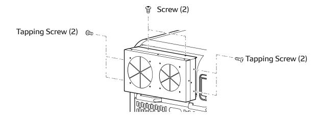
8. Attach the cold air flange to the adapter with the four (4) screws.
