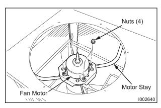
**4)** Take off the four (4) nuts, and then remove the condenser fan motor.
