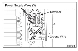
2) Disconnect the three (3) power supply wires from the terminal, and disconnect the ground wire.
