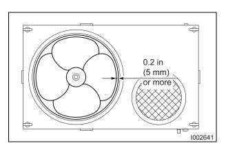
• Install condenser fan. Allow a clearance of 0.2 in (5 mm) or more on side of the condenser fan.
