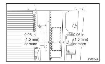
Install evaporator fan. Allow a clearance of 0.06 in (1.5 mm) or more on side of the evaporator fan.
