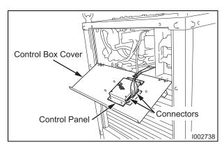
**1)** Disconnect the two connectors (11-pin, 5-pin) from the control panel.
