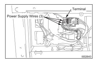
1) Disconnect the three (3) power supply wires from the terminal.
