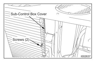
1) Take out the two (2) screws, and then remove the sub-control box cover.
