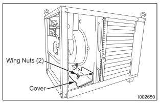
**3)** Take off the two (2) wing nuts, and then remove the cover.
