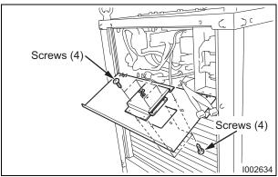
**2)** Take out the eight (8) screws, and then remove the control panel.
