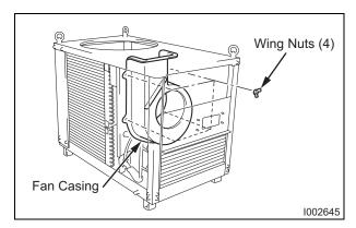
**4)** Take off the four (4) wing nuts, and then remove the evaporator fan casing.
