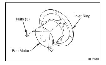
**5)** Loosen the set bolt using a box wrench, and then remove the evaporator fan.
