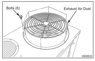
**7)** Take out the six (6) bolts, and then remove the exhaust air duct.
