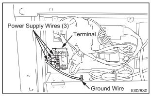
**4)** Disconnect the three (3) power supply wires from the terminal, and disconnect the ground wire.
