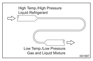
the fixed orifice in the capillary tube. As a result, the temperature and state of the refrigerant becomes low and mist-like, and therefore evaporates easily.
