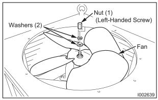
**3)** Take off the nut (left-handed screw) and two (2) washers, and then remove the condenser fan.
