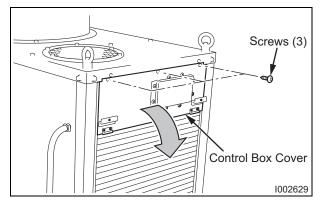
**3)** Take out the three (3) screws, and then open the control box cover.
