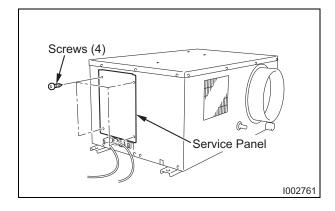
**1)** Take out the four (4) screws, and then remove the service panel.
