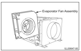
2) Disconnect the motor connector (white, six-pin) from circuit board CN23, and remove the evaporator fan assembly.
