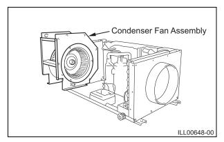
2) Disconnect the motor connector (white, six-pin) from circuit board CN22, and remove the condenser fan assembly.
