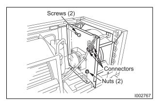
Disconnect the three connectors (two white, twopin connectors; one white, three-pin connector), and then take out the two (2) screws and the two (2) nuts.
