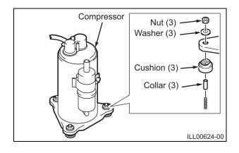
Install three (3) cushions and three (3) collars to the bolts and mount the supplied compressor to the unit.
