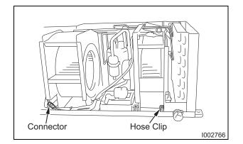
**3)** Take out the eighteen (18) screws, and then remove the top panel.
