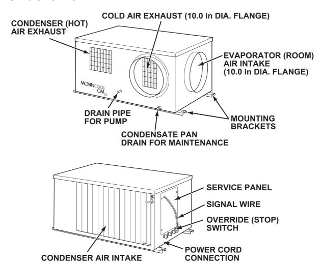
MARNING: Remove protective cardboard from condenser intake after installation.
