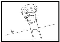
Position the clip to the top of the drain pipe near the unit as shown.
