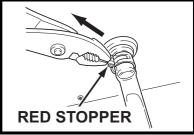
3. Pull out the red stopper and secure hose. Make sure there are no kinks or bends. When using the gravity drain, make sure the hose is connected as a decline.
