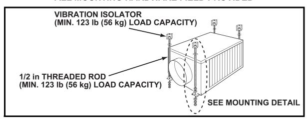
Install the four field-supplied rods by suspending them from suitable building structure members. Locate the rods so that they will align with four mounting holes in the mounting bracket that are part of the unit base.
