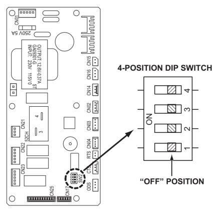
The CM12's controller is equipped with a 4-position DIP switch, which defaults in the OFF position. The DIP switch can be set to configure the following functions:
