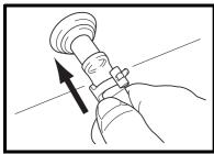
1. Plug in the 1/2 inch (13 mm) drain hose with the lose clip into the drain pipe. Make sure the hose is all the way in and flush with the grommet.
