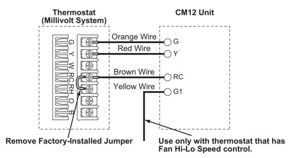
Note: Use thermostat that is compatible with millivolt system. Do not connect thermostat to AC power source.
