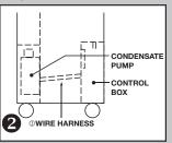
From the rear of the Movin-Cool unit, locate the ①wire harness that was previously passed through the grommet. ①=adapter
