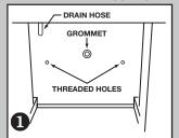
Place the Condensate Pump in the compartment of the previously removed drain tank. Pass the adapter wire harness through the grommet.
