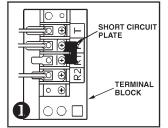
From the control box, remove the short circuit plate from the terminal block.
