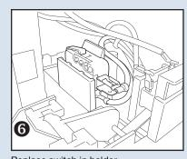
Replace switch in holder. Note: Retaining tab should be on top of switch.
