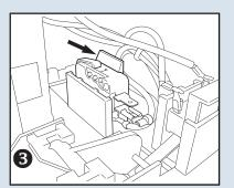
Remove main switch assembly from holder by pushing retaining tab and lifting switch.
