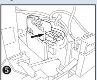
Reattach wire to top terminal of main switch. Check resistance across top and bottom terminal (should be "closed"). Lift float to confirm proper switch operation (should be "open").
