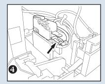
Locate and disconnect wire which is connected to the middle terminal of the main switch.
