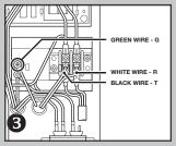
terminal lead wires to the terminal block spade connectors located in the control box.
