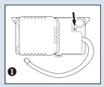
Remove cover secured by screw.
