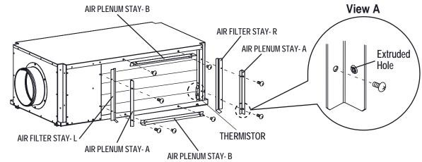
4. Insert the air filter into the condenser intake of the unit, and make sure the filter tap is located at the bottom side.
