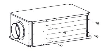
3. Install Stay - L and Stay - R with four (4) screws which were previously removed. Note: Be careful not to damage the thermistor when installing Stay - R.
