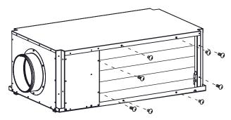
3. Install both Stay - A with four (4) L10 screws and both Stay - B with four (4) L6 screws which were previously removed.
