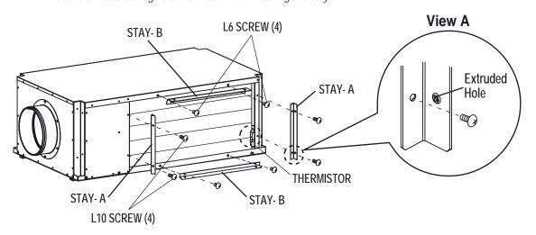
4. Install the assembled air plenum to the installed stays with the supplied eight (8) screws.
