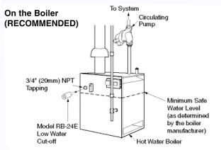
2. If no tapping is provided on the boiler, the probe control can be installed in a header or riser pipe above the boiler. Refer to the Typical Installation Diagrams below.
