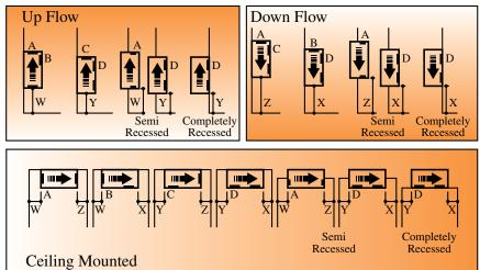
KEY: W = 6" minimum, X = 12" minimum, Y = 0" or greater, Z = 24" minimum front to provide access to mounting holes.
