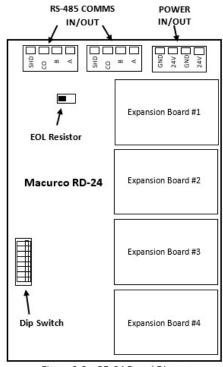
Figure 3-3 - RD-24 Board Diagram
