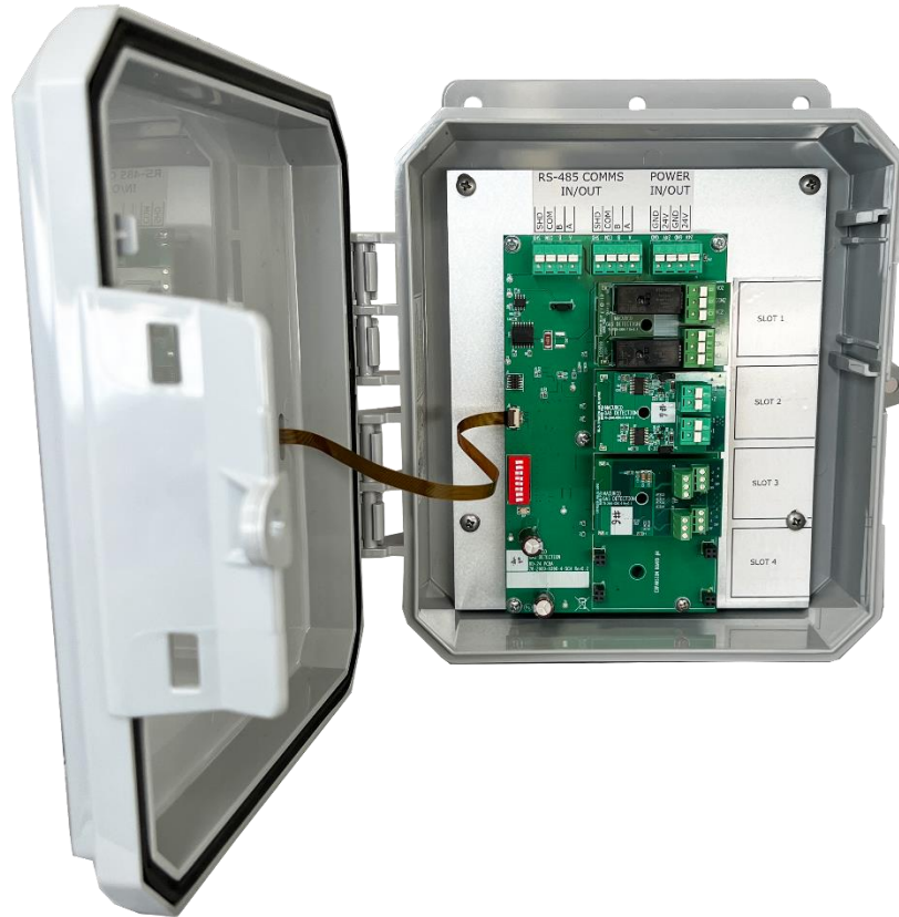
Figure 3-2 – Internal view with expansion boards
