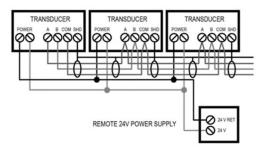
Figure 3-3 Modbus Wiring
