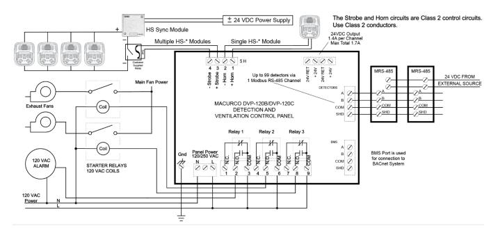
Figure 3-3 System Wiring Diagram
