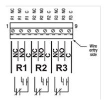
Figure 3-7 Relay Connector
