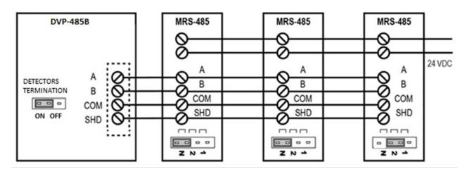
Figure 3-13 EOL Placement greater than 1000 ft
