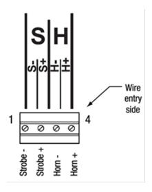
Figure 3-8 Horn & Strobe Connector
