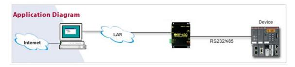
Figure 5-3 RS-485 to Ethernet (TCP/IP)
