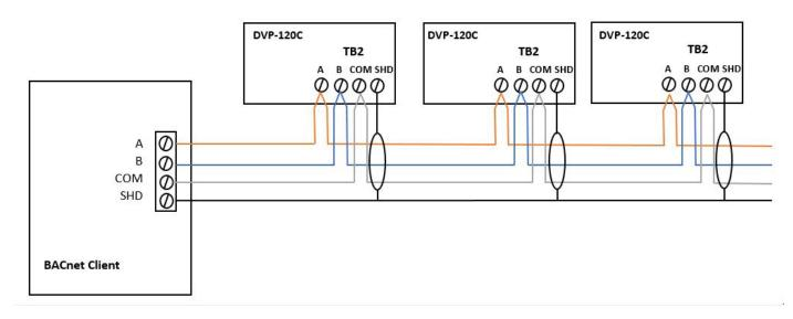
Figure 5-3 BACnet Connection
