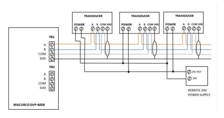
Figure 3-10 Modbus Wiring
