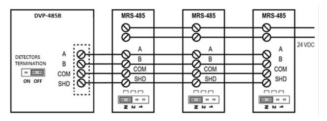
Figure 3-12 EOL Placement Less than 1000 ft
