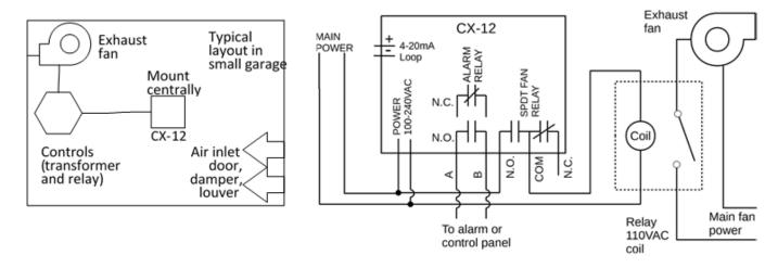
Figure 3–13 12-Series Typical Installation
