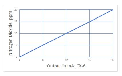
Figure 3–2 6-Series 4-20 mA NO2 Output diagram
