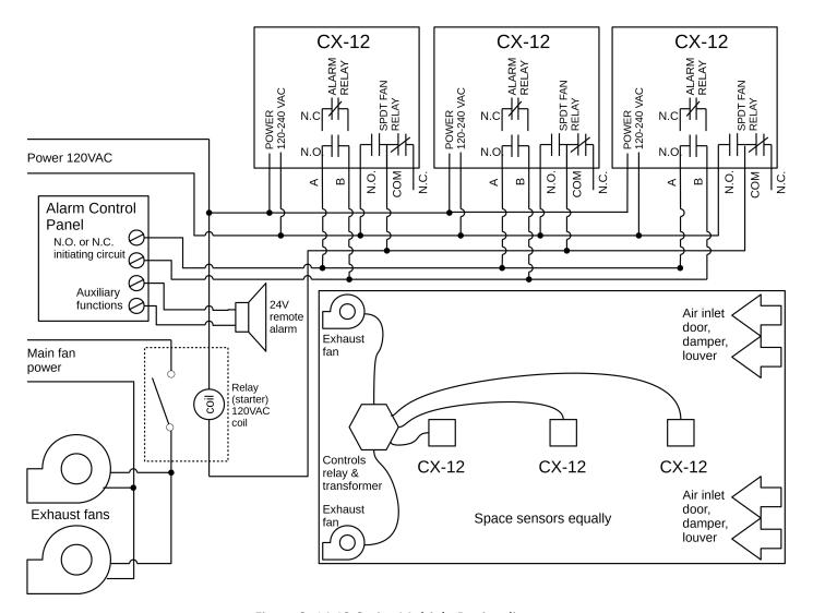
Figure 3–14 12-Series Multiple Device diagram
