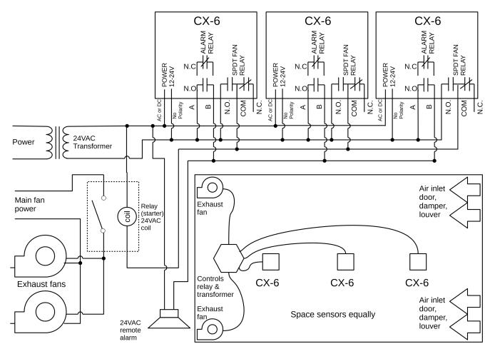
Figure 3-5 6-Series Multiple Devices
