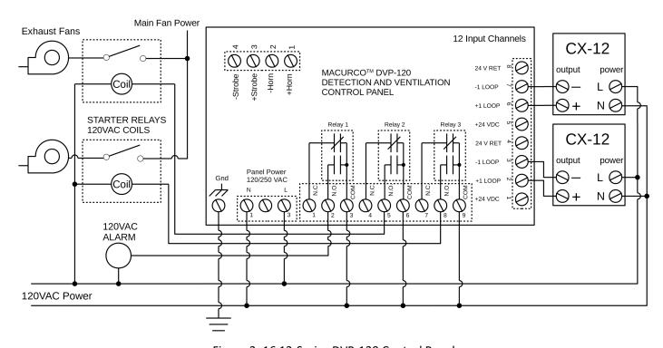
Figure 3–16 12-Series DVP-120 Control Panel
