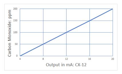
Figure 3–10 12-Series 4-20 mA CO Output diagram
