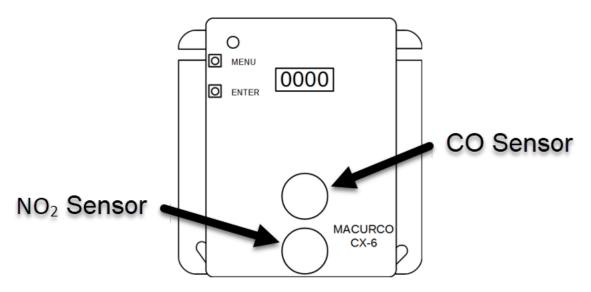
Figure 5-3 - Replacement Sensor Location
