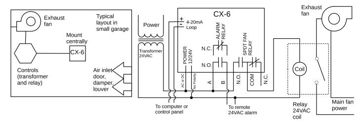
Figure 3–4 6-Series Typical Installation
