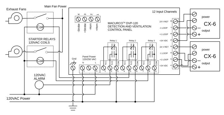
Figure 3–7 6-Series DVP-120 Control Panel
