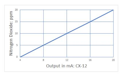
Figure 3–11 12-Series 4-20 mA NO2 Output diagram
