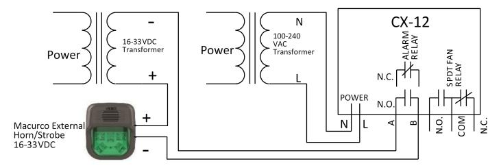
Figure 3-18 12-Series Horn & Strobe Combo Wiring
