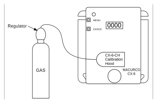
Figure 7–1 - Calibration Kit Connection
