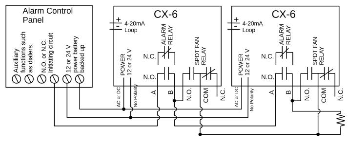
Figure 3-8 6-Series Alternate Alarm Panel
