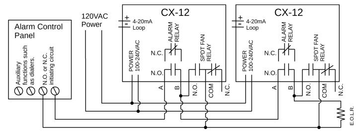
Figure 3-17 12-Series Alternate Alarm Panel
