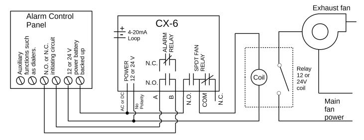
Figure 3-6 6-Series Alarm Control Panel
