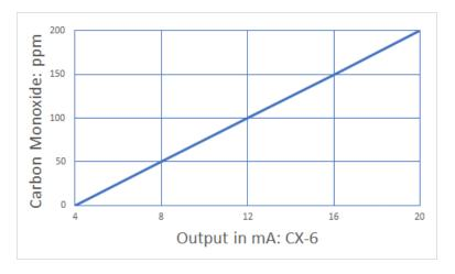
Figure 3–1 6-Series 4-20 mA CO Output diagram
