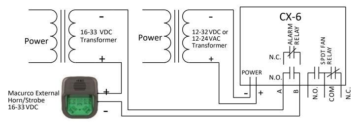
Figure 3-9 6-Series Horn & Strobe Combo Wiring
