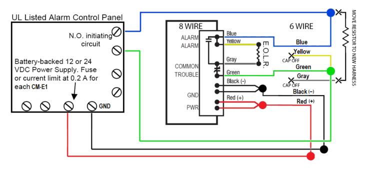
Figure C-3 – 6 pin to 8 pin wiring diagram.
