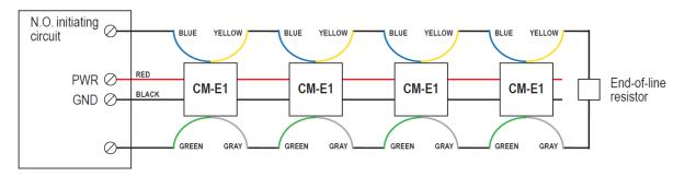
Figure 3-2 – Series Wiring
