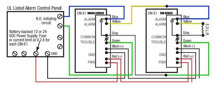
Figure 3-3 – Typical Connection of two CM-E1's in series to an alarm control panel
