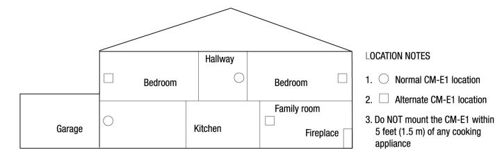
Figure 3-1 – Typical Install Locations
