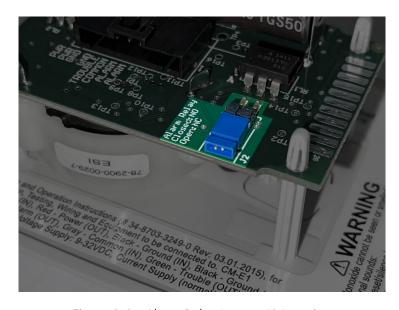
Figure 3-6 – Alarm Relay Jumper J2 Location
