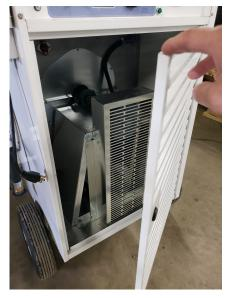
Locate the face plate and remove the screws and nuts to expose the connector slot on the heater. Save the screws and nuts. See Fig. 2.
