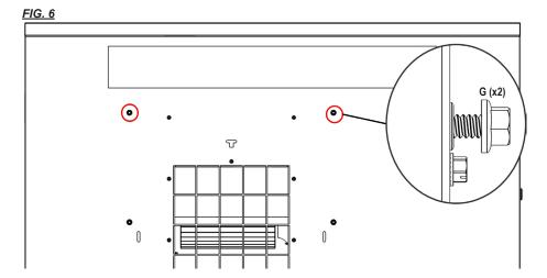
Lift the duct adapter assembly and align the top holes to the previously installed screws (G) as shown in FIG. 7.
