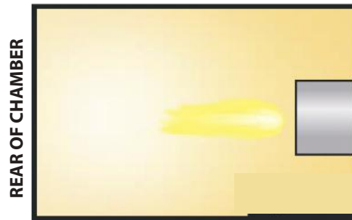
Flame is under-fired
