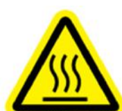
Burn Hazard / Hot Surface
