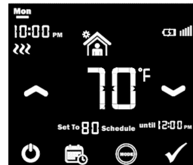
Low Battery Indicator
