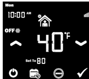
Freeze Protection Off (Heat Turns On When Room Drops Below 40F)
