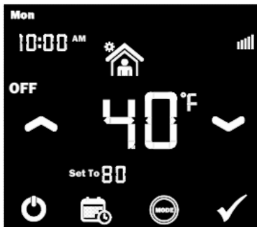
System Off (Heat Stays OFF Regardless of Room Temp)
