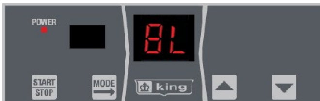
Heater Display – Heater Locked Out
