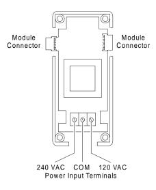
Figure 3: Interior of the Y350R Power Module
