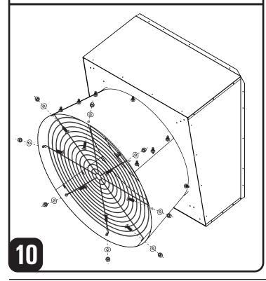
After guard is installed apply the ratchet strap around the cone near the venturi and tighten until no gaps appear between the venturi and the cone. Once the cone is effectively contracted, tighten the slotted truss head screws that connect the cone panels together. After all screws are tightened remove ratchet strap.
