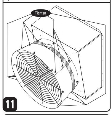
Swivel top and side shutter clips open. Set bottom shutter flange between housing flange and bottom shutter clips. Secure shutter by swiveling top and side shutter clips over shutter flange.
