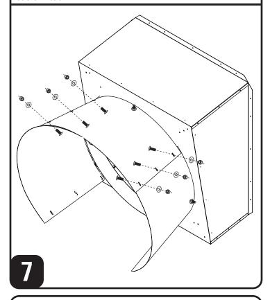
Attach bottom cone section to the venturi like you did the top and side cone sections in <u>Steps 6 and 7</u>. The bottom cone section should rest inside of the side cone sections to help shed water.
