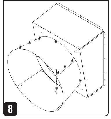
With the bottom cone section inside the side cone sections, fasten sections together using (6)  $\frac{1}{4}$ " x  $\frac{3}{4}$ " slotted bolts with (6)  $\frac{1}{4}$ " washers and (6)  $\frac{1}{4}$ " nylock nuts, but DO NOT TIGHTEN .
