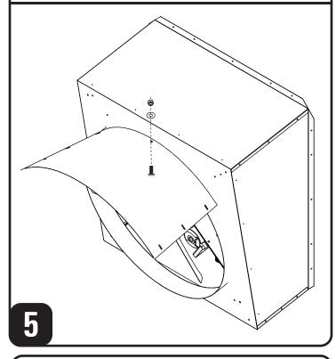
Attach both side cone sections to the venturi like you did with the top cone section in **Step 6**. The top cone section should overlap the side cone sections to help shed water.
