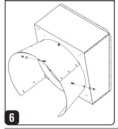
With the top cone section overlapping the edges of the side cone sections, fasten sections together using (6)  $\frac{1}{4}$ " x  $\frac{3}{4}$ " slotted truss head screw with (6)  $\frac{1}{4}$ " washers and (6)  $\frac{1}{4}$ " nylock nuts, but DO NOT TIGHTEN.
