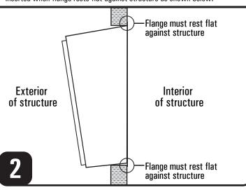
Center the fan body in wall opening. Using the holes indicated, secure fan to framework with (12) fasteners (not provided) suitable for your structure.
