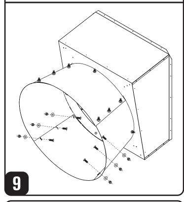
Fasten guard to cone using (8)  $\frac{1}{4}$ " x  $\frac{3}{4}$ " slotted truss head screw with (8)  $\frac{1}{4}$ " washers and (8)  $\frac{1}{4}$ " nylock nut.
