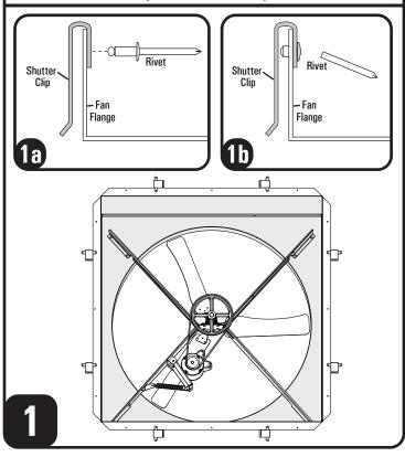
Lift and tilt fan body as you insert fan into the rough opening. Fan is fully inserted when flange rests flat against structure as shown below.
