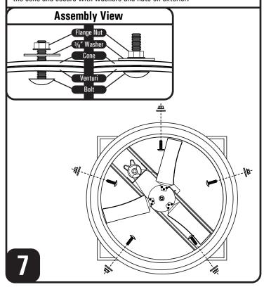
Place guard against cone flange. Using 5/16" drill bit and the guard mounting feet as guides drill holes through the cone flange. Secure the guard to the cone using (8) 5/16" carriage bolts, (8) 5/16" flat washers, and (8) 5/16" nylock flange nuts. Review the Assembly View illustration for proper installation. Do not tighten until all have been assembled.
