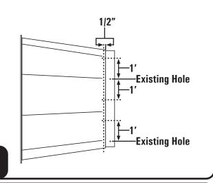
Using the lines made in  $\underline{\text{Step A}}$  as your guide and a 3/8" drill bit, drill a hole through the cone as shown below.
