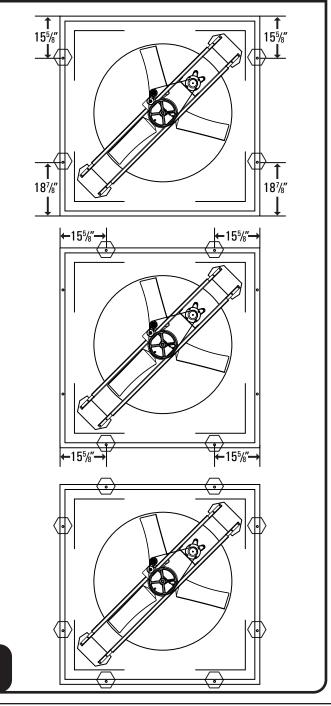
Attach all (8) shutter clips with a rivet gun using (8) 3/16" rivets and (8) 3/16" washers. Review the illustrations below for placement and assembly.
