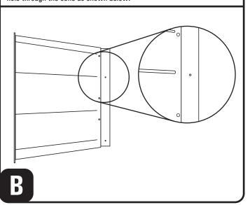
Using a circular saw cut slit connecting the edge of the mounting ridge to the hole drilled in  $\underline{\text{Step B}}$  as shown below.
