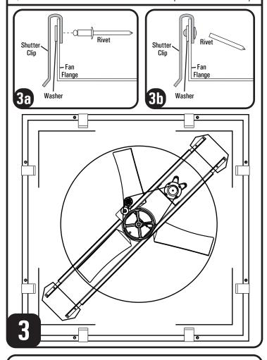
From the inside of your structure, rotate the fan housing until the motor is located above and to the right of the shaft, as shown below. Insert fan housing into the finished opening and secure all 4 sides to structure using suitable fasteners and washers (not included).
