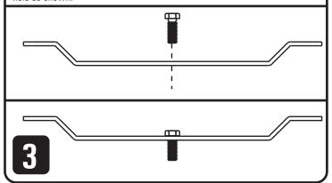
Attach the Installation Bracket to your structural beam or stud using hardware (not provided) that is capable of supporting 150 lbs (68 kgs).
