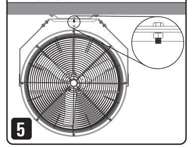
Now that your Poly Chiller is securely installed to your structure, you may remove the (1) 3/8" · 16 x 1·1/4" Hex Bolt and (1) 3/8" · 16 Nylock Nut installed in the top tilt position in each Side Hanging Bracket in Step 1.
