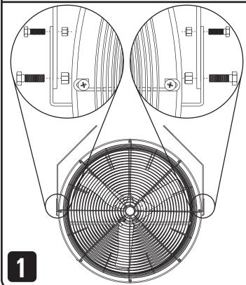
Attach the Top Hanging Bracket to the Side Hanging Brackets as shown using (4)  $5/16'' \cdot 18 \times 1''$  Carriage Bolts and (4)  $5/16'' \cdot 18$  Nylock Flange Nuts
