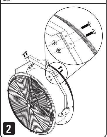
IMPORTANT!! Before attaching the Installation Bracket to your structure, you must insert (1) 1/2" - 13 x 1-1/2" Hex Bolt into the center mounting hole as shown.
