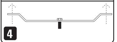
Once the Installation Bracket is secured to your structure, lift and attach the Poly Chiller to the Installation Bracket by inserting the (1)  $1/2'' - 13 \times 1-1/2''$  Hex Bolt through the hole in the Top Hanging Bracket. Secure using (1) 1/2'' - 13 Nylock Nut.
