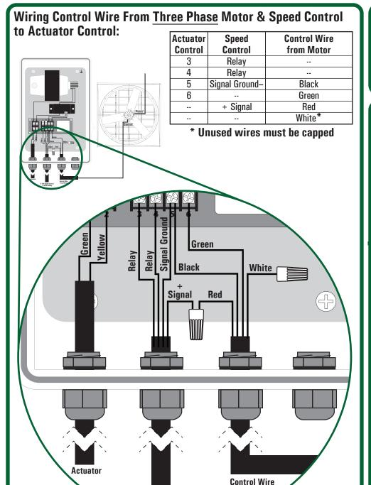
0-10V Speed Control & On/Off Relay From Motor
