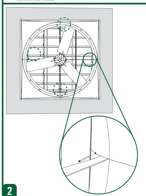
To further secure and prevent water, condensation, and ice from penetrating, use a sealant (Minimal-Expanding Foam / Polyurethane Caulk) on all four sides to fill the gaps between the housing and the rough opening.
